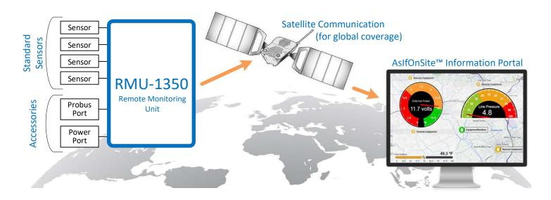
Proactive Sensing made the installation and configuration of the RMU-1350 remote monitoring system both simple and intuitive. Just choose the parameter template from our solution library that best suits your application, customize a few settings to your specific requirements, connect an industry-standard sensor, and start receiving detailed tracking and monitoring information through the AslfOnSite information portal.
